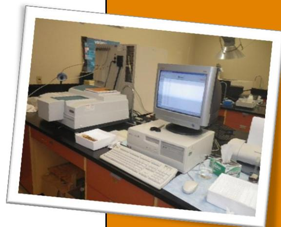
Measuring maple syrup colour and total phenolics using a UV/Vis spectrophotometer at Dalhousie University
